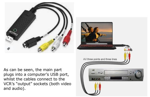
We all know that the quality of VCR videos is, these days, very poor compared with modern TVs and computer monitors, but it may be possible to improve the quality depending on the output port types on the video player being used (Composite vs Component vs S-Video, and L/R audio vs single cable) ... essentially, the more cables used, the better.
