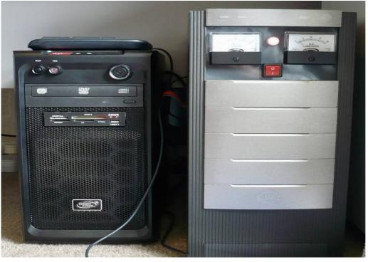
The second is a photo of a recycled Quay Computer case containing the 13.8 Volt 20 Ampere power supply for the transceiver.
